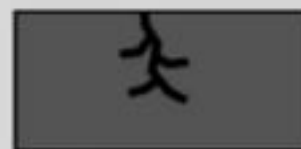
Stress Corrosion Cracking
