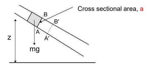
An element of fluid, as that in the Fig., has potential energy due to its heights z above a datum and kinetic energy due to its velocity V. If the weight is mg then,
