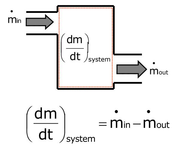
For steady state flow, there is no increase in the mass with in the control volume/chosen boundary, means  $(dm/dt)_{system} = 0$
