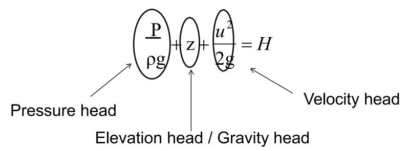
By the principle of conservation of energy the total energy in the system does not change, Thus the total head does not change. So the Bernoulli equation can be written
