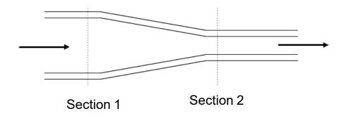
Discharge at Section 1 = discharge at section 2  $\rho_1 \, Q_1 = \rho_2 \, Q_2 \, ( \text{ if consider incompressible fluid} )$  so,  $A_1 u_1 = A_2 u_2$   $u_1 \, d_1{}^2 = u_2 \, d_2{}^2$
