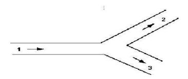
Total mass flow into the junction = Total mass out of the junction  $\rho_1 Q_1 = \rho_2 Q_2 + \rho_3 Q_3$
