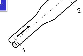
total energy per unit weight at 1 = total energy per unit weight at 2
