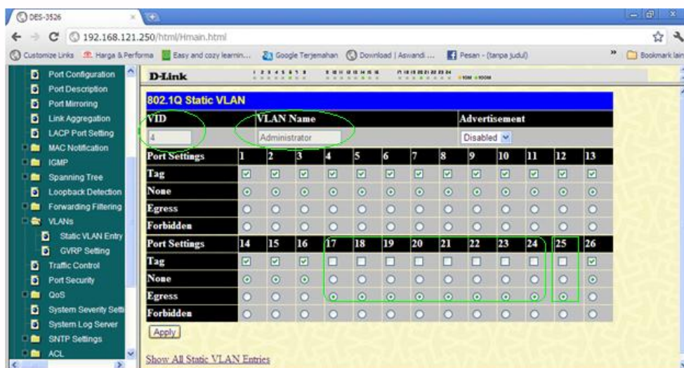
Gambar 4.24 Konfigurasi Grup VLAN (VID 4, VLAN Name Administrator, Port 17-24 & 25)
