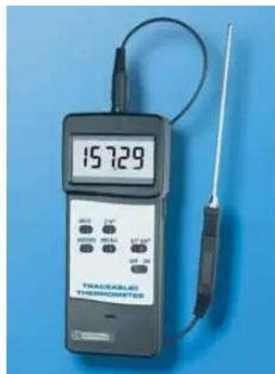
**Gambar 8.2** Termometer hambatan listrik
