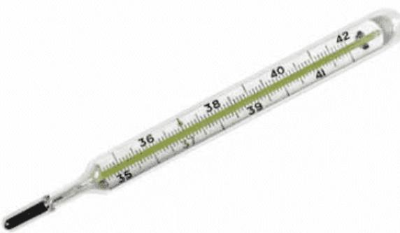
**Gambar 8.1** Termometer Zat Cair
