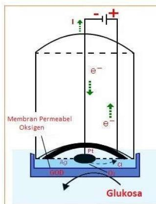
**Gambar 5.6** Biosensor Amperometrik
