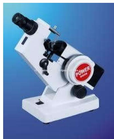
**Gambar 2.28** Alat Lensometer
