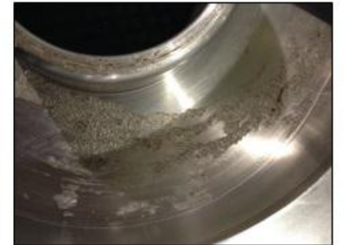
Pitted erosion caused by cavitation. Source: hollandaptblog
