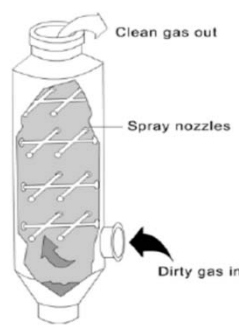
Counter current spray tower (Sumber: APTI, 1999)
